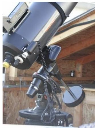
With the focuser modification complete it was now time to make the focusing function controllable from the observatory computer. This was achieved using a FCUSB (USB= Universal Serial Bus) focus controller from Shoestring Astronomy. I also ordered a GPUSB auto guider interface which I haven't yet got hooked up and running.
